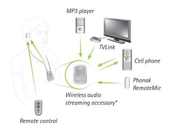
\* Audio sources can be connected by Bluetooth® or cable to the wireless audio streaming accessory.
