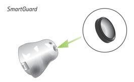
Cerustop wax guards are also commonly used as an alternative protection system. Your hearing care professional will provide you with detailed information on the use of the wax protection system on your hearing aid.
